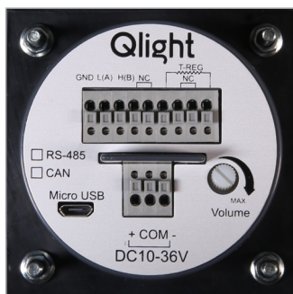
Terminal box for Signal phone for CAN communication panel (back side)
